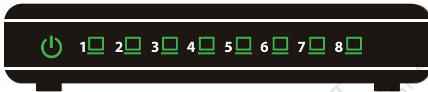
Figure 10.11: A network hub with 8 ports
